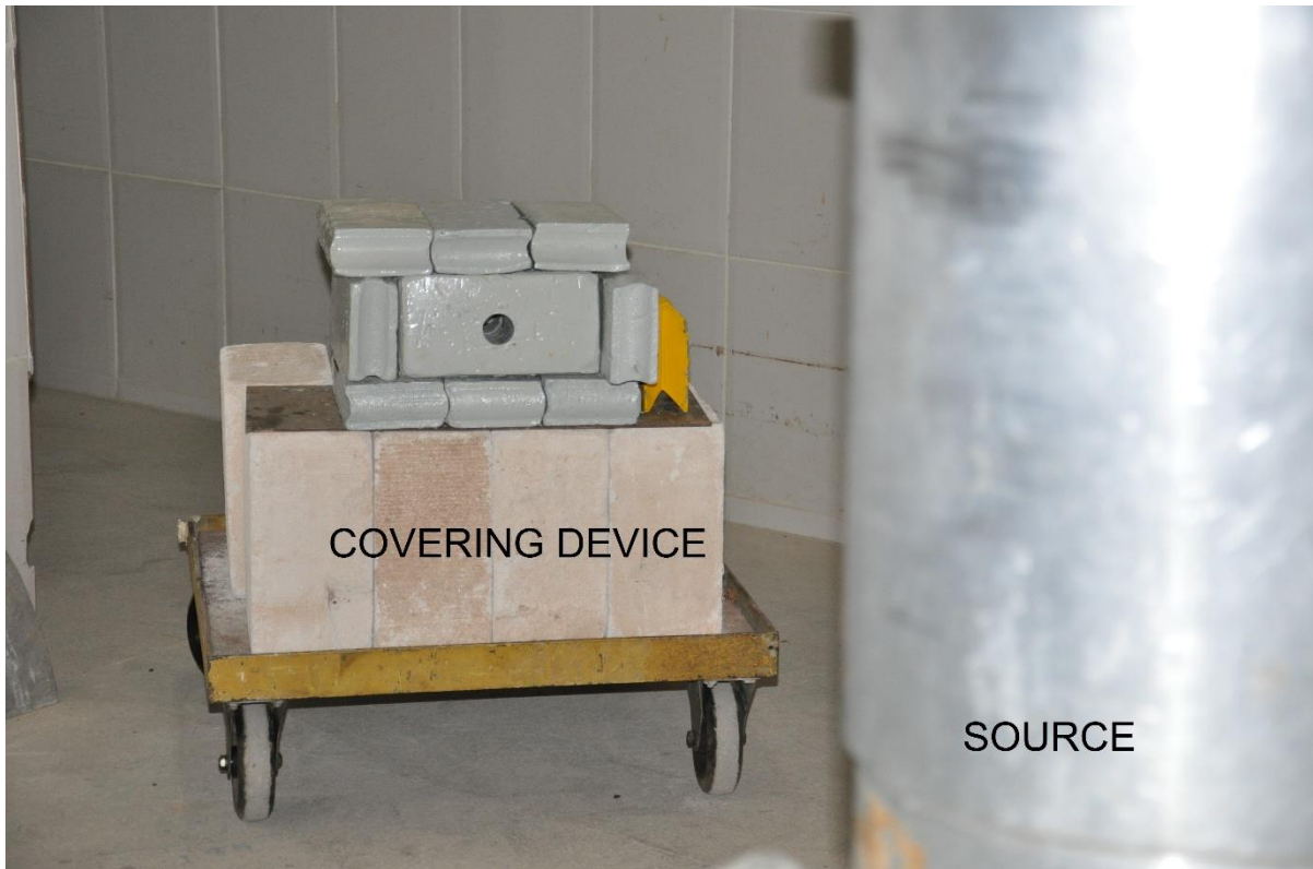
Figure 2 - Protection plumb device and collimator around the source.
