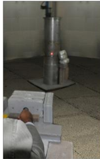
Figure 4 - Laser used to determine the beam axis.
