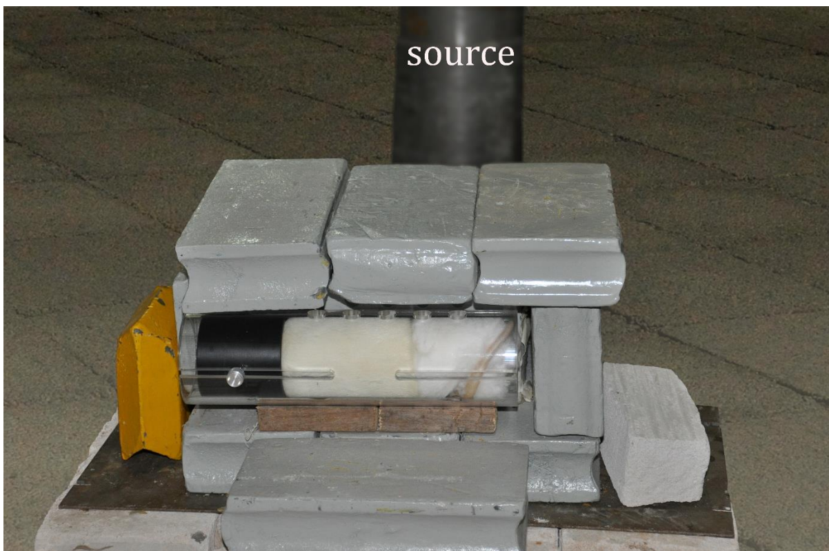
Figure 3 - Rat protected with a covering device at a 2m distance from the source.
