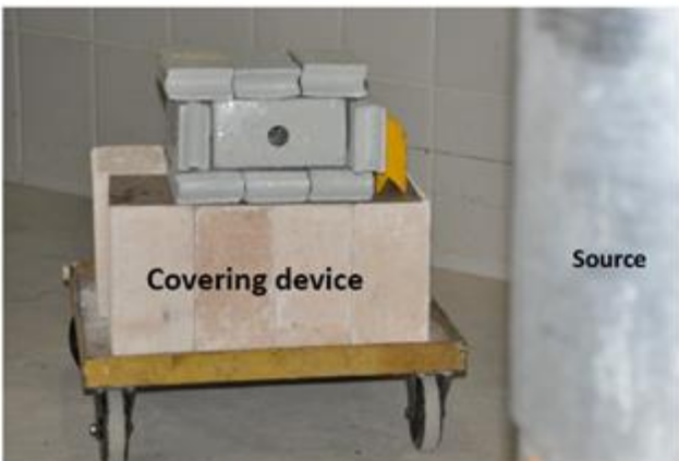
Figure 2 - Covering device and collimator at a 2m distance from the source.
