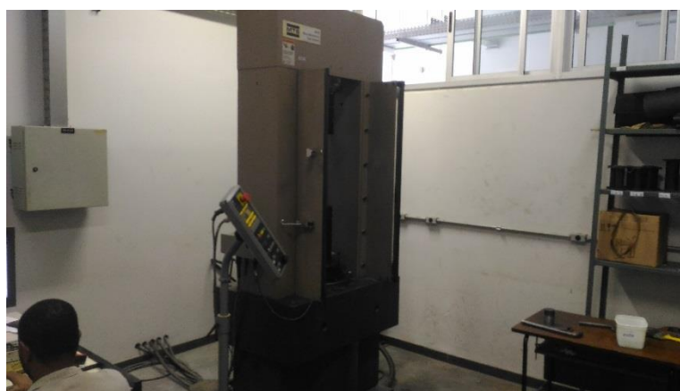
Figura 32 – Prensa MTS Systems Corporation - Rock Mechanics Test system, Model No. 315.02, Force: Comp 2853 KN). Fonte: Autor (2018)
