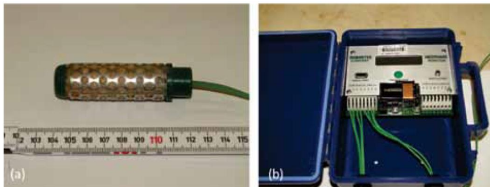
Figura 18 – (a) Sensor de matriz granular. (b) Datalogger Watermark Monitor 900M (Marinho et al. , 2015).
