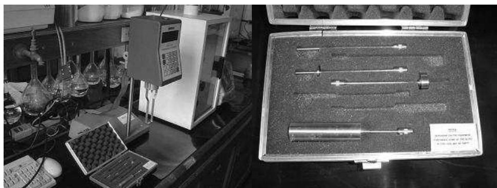
Figura 4.13: Viscosímetro Brookfield, modelo DV-III. ( www.brookfieldengineering.com ).
