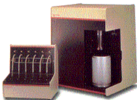
Figura 4.5: Unidade Tristar Nitrogen Adsorption. ( www.particletechlabs.com )
