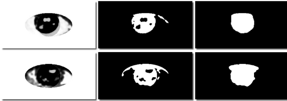
Figure 3.8. Each row shows the image ROI for the black iris and the blue iris showed in Figure 3.7. The first column shows the ROI after the mask subtraction, the second column shows the result the binarization result, and the last column shows the final result after hole filling and morphological operations.
