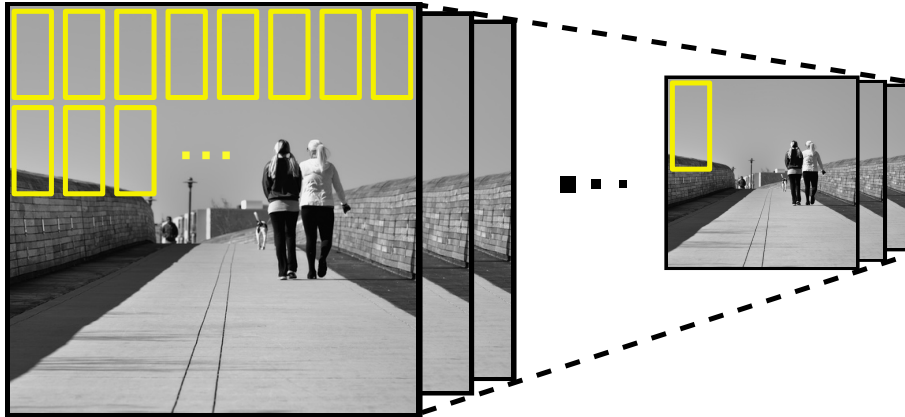
Figure 3.2. Sliding window algorithm. The input image is scanned in all possible locations and in multiple scales by a detection window, whose size is kept fixed in our work. This example illustrates non-overlapping windows, but real systems sets the strides such that the windows overlap with each other, avoiding to skip a pedestrian.
