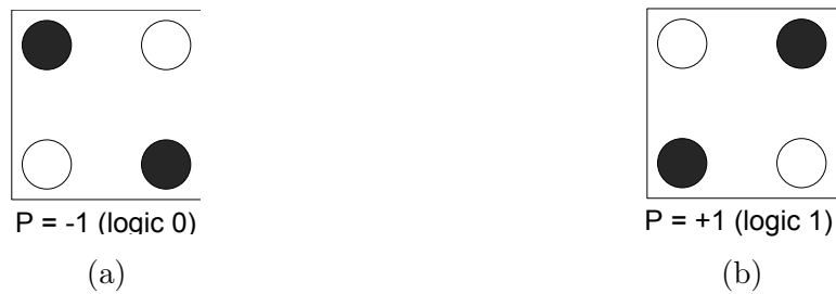
Figure 2.1: QCA cells on the two possible states. (a) Polarization P = -1 represents a logic 0 and (b) P = +1 represents a logic 1. Squares' edges represent the cell boundaries where exists a high potential barrier and circles represent quantum dots. Black circles are quantum dots containing electrons
