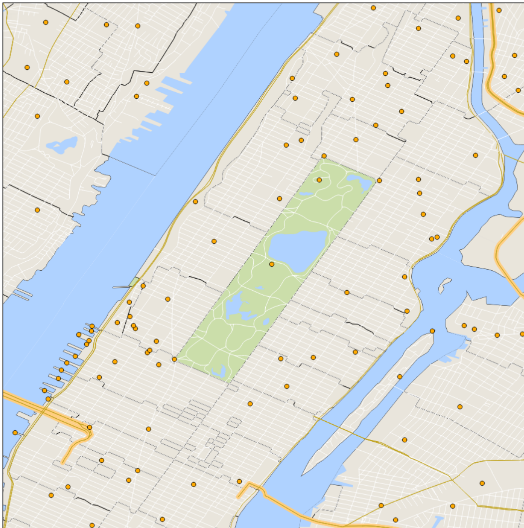
Figure 4.1: 2013 TIGER/Line collections AREALM, AREAWATER, ROADS, PRISE-CROADS, PRIMARYROADS and POINTLM at the Manhattan's Central Park.
