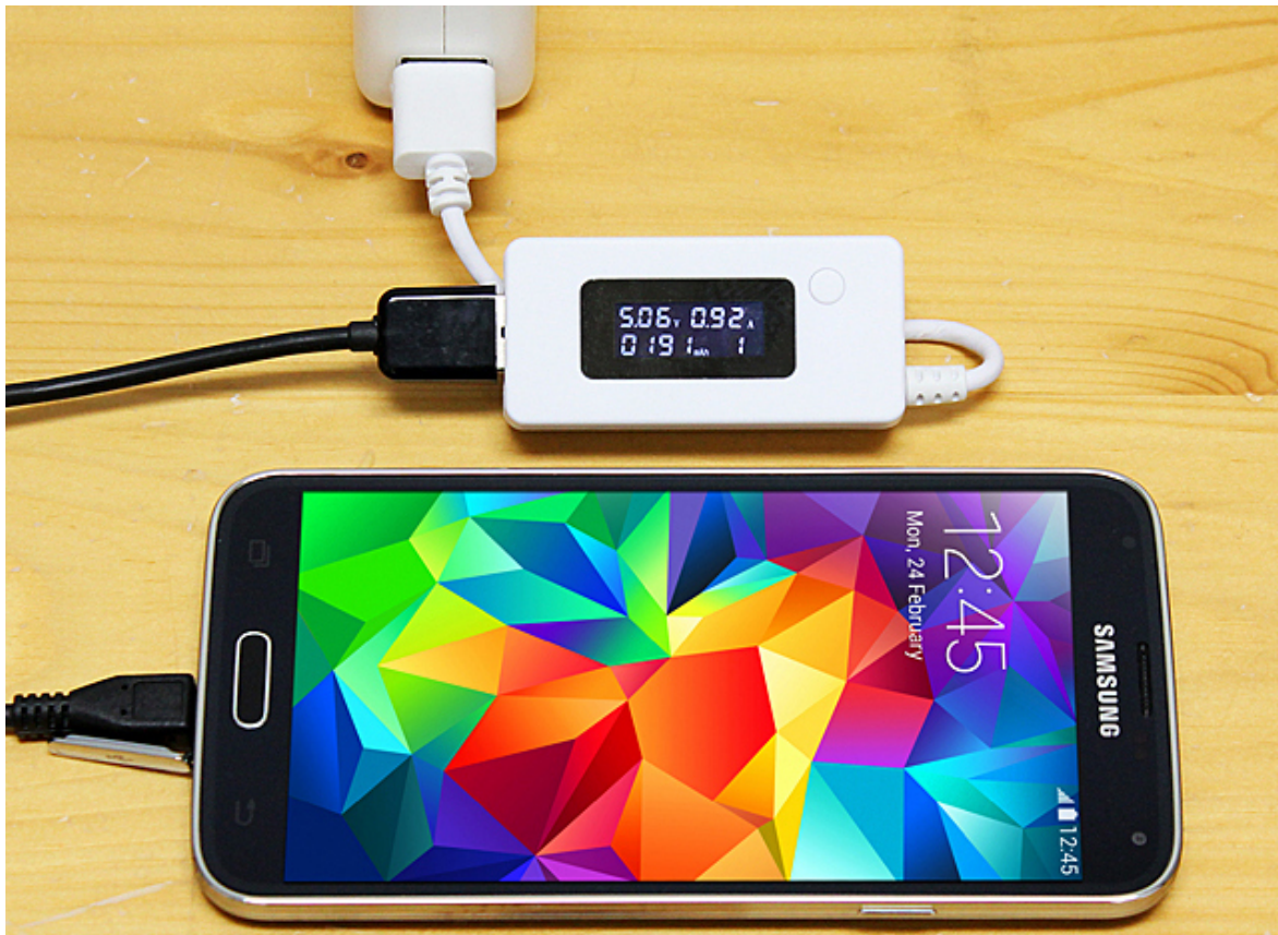
Figure 4.4. KCX-017 - Measuring the phone's energy consumption
