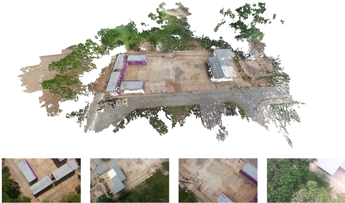
Figure 1.1. DEM reconstructed by our pipeline followed by a sample of 4 images out of 220 used in the estimation from a construction site near ICEX. The model was obtained with minimal budget using a smartphone camera and a low-cost quadrotor.
