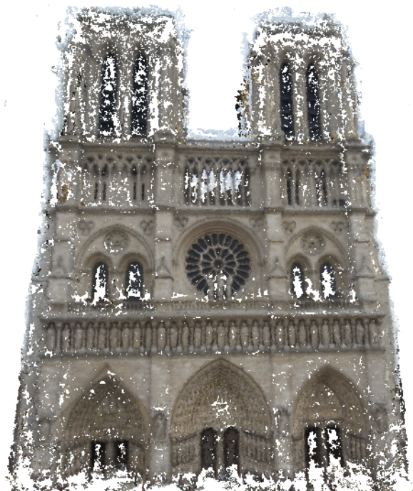
Figure 5.9. Result of the “Notre Dame” dataset experiment. Our methodology estimate this model with a re-projection error of 0.43 spending 27.4 hours, while Bundler returned an error equal to 0.47 and 86.7 hours of processing.
