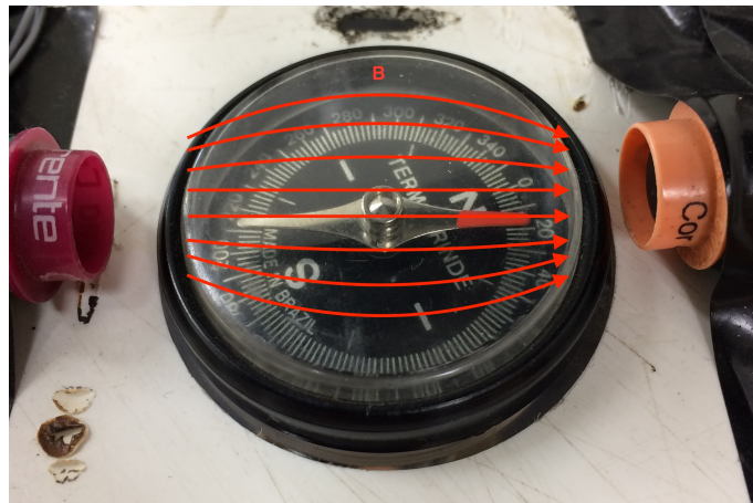
Figure 4.3. Magnetic field using the electronic system. In this image the coils generate a magnetic field B from the left to the right, as shown by the red arrows. Note that the compass aligns with the magnetic field lines.
