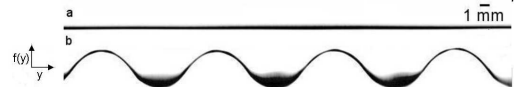
FIG. 2: Images of the straight(a) and periodic(b) morphologies of the interface. In both images the open atmosphere is located above the interface and silicon oil is located below the interface. Experiments set for b_o = 400\mu\text{m} and \omega = 4.85\text{rad/s} (a) and \omega = 5.39\text{rad/s} (b).
