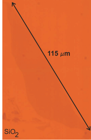
Figure 4.5: Graphene on top of a silicon substrate with a silicon oxide layer of 300 nm thickness. The picture was taken in a optical microscope with a red filter to enhance even more the contrast.
