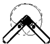
X-Y miking employs a matched pair of coincident cardioids
