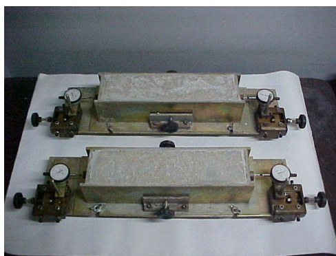
Figure 9. 1 – Autogenous shrinkage test
