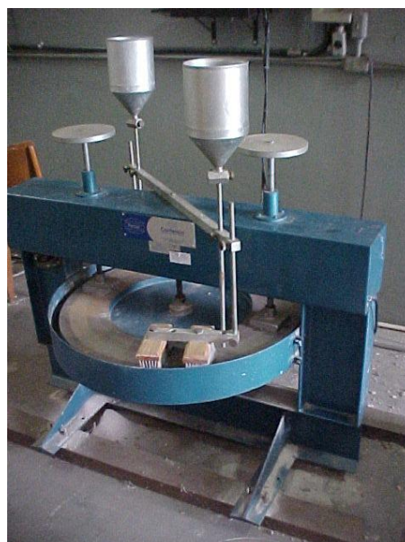
Figure 6. 2 – Surface wearing machine for abrasion resistance of concrete.
