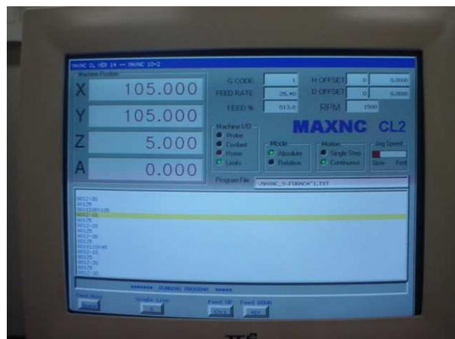
**FIG. 4.17–** Interface do *software MaxNC*.
