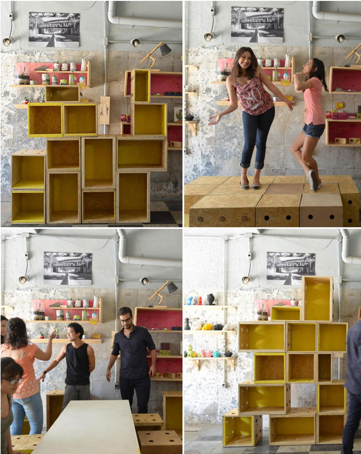
Figure 21 | Several combinations of the 13 modules assembled by the students (shelve, stage, bench, table, and others). The modules were built in 3 sizes: small, medium, and large. (author, 2016).
