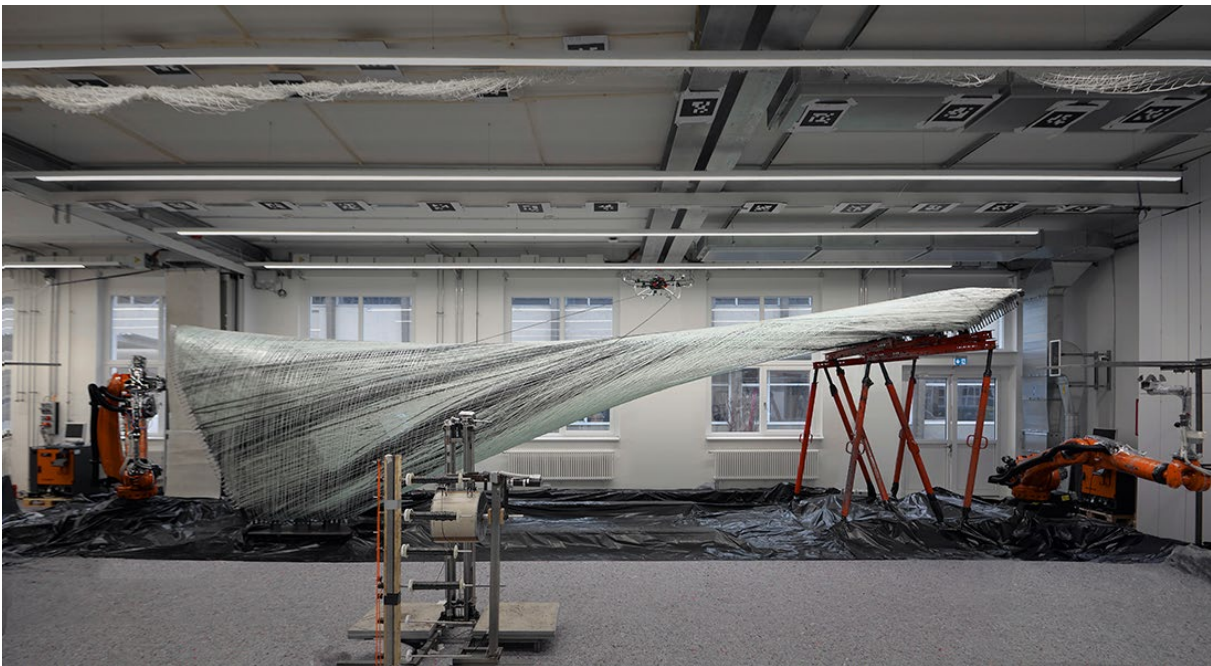
Figure 42 | Research pavilion by The Institute for Computational Design and Construction (ICD) and the Institute of Building Structures and Structural Design (ITKE) at the University of Stuttgart exploring building-scale fabrication of glass and carbon fibre-reinforced composites. ("ICD/ITKE Research Pavilion 2016-17 | Institute for Computational Design and Construction," 2017)
