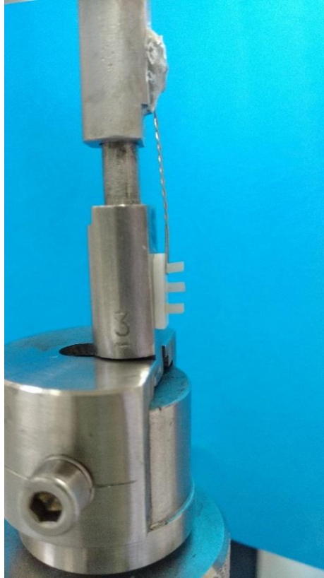
Figure 3: Specimen coupled to the universal testing machine (EZ Test - S Shimadzu, Tokyo, Japão).
