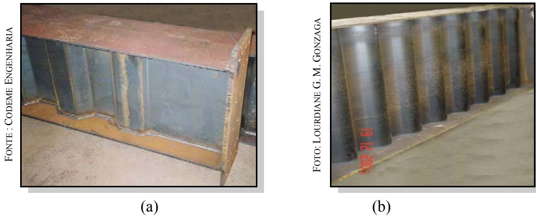
FIGURAS 1.1 – Perfis com alma corrugada (a) trapezoidal (b) senoidal
