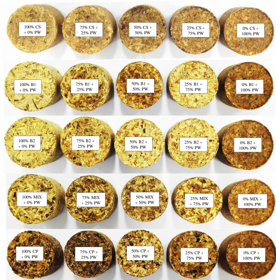
Fig. 2. Briquettes produced with different mixtures of residues. PW = Pine Wood. CS = Coffee Stem. B1 = Primary Branch. B2 = Secondary Branch. Mix = Stem + Primary Branch + Secondary Branch. CP = Cherry Parchment.
