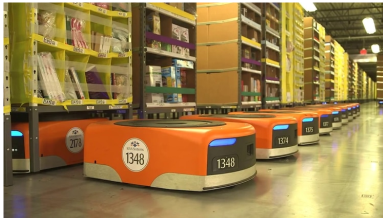
Figure 1.2. Multiple robots that transport stacks of products at Amazon warehouse. Source: www.infobae.com
