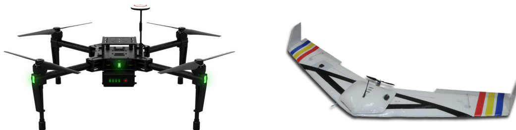
Figure 1.3. On the left is a quadrotor DJI Matrice 100 ( Source: https://store.dji.com ). On the right is a fixed-wing UAV developed at UFMG.
