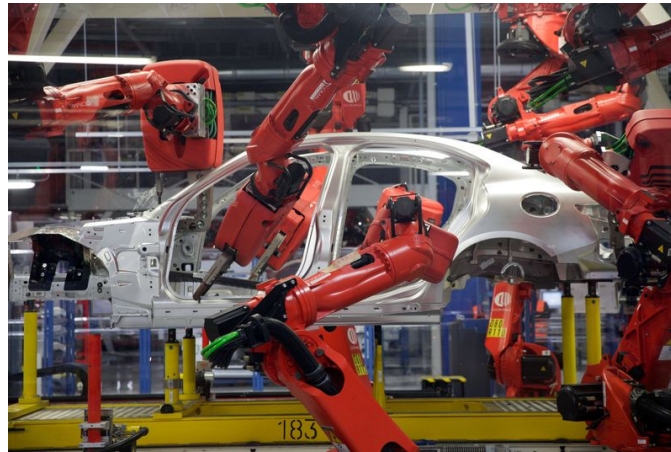
Figure 1.1. Multiple robotic manipulators, manufactured by Comau, working on an automobile on the production line at Fiat Chrysler Automobiles. Source: https://www.bloomberg.com .
