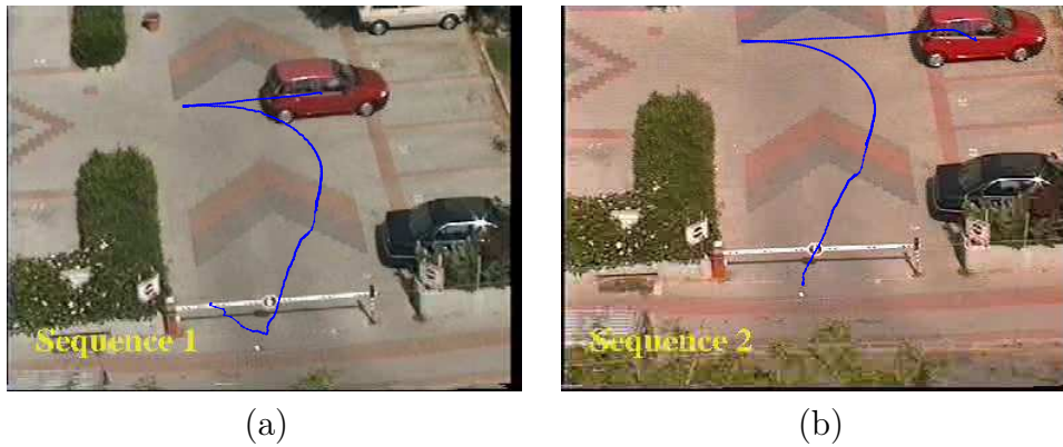
Figure 3.2: (a) Trajectory of the car’s pixel centroid in Sequence 1. (b) Trajectory of the car’s pixel centroid in Sequence 2. The car was tracked by a simple blob tracker that relies on foreground-background detection to label all foreground pixels in each frame.
