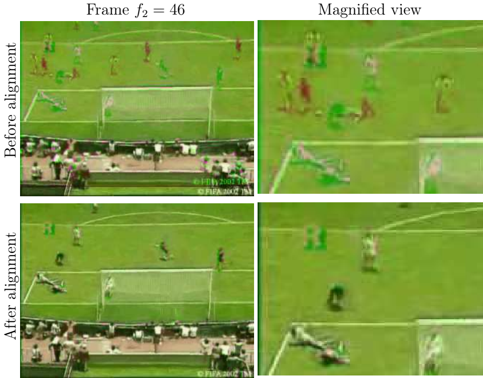
Figure 5.11: Before alignment images were created by superimposing the green band of a frame f_2 with the red and blue bands of frame f_1^* = (f_2 - \beta^*)/\alpha^* using ground truth timeline coefficients \alpha^* and \beta^* . After alignment images were created by replacing the green band of the images above them with that of frame f_1 = (f_2 - \beta)/\alpha , with \alpha, \beta computed by our algorithm. For both types of images, deviations from the ground-truth alignment cause “double exposure” artifacts (i.e., when f_1^* \neq f_2 or f_1^* \neq f_1 , respectively).
