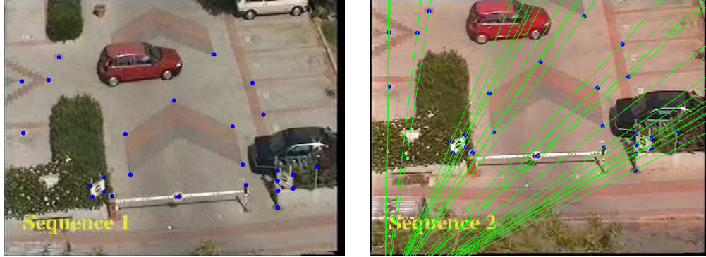
Figure 5.2: The recovered epipolar geometry for the two-view Car dataset. Points and their epipolar lines are displayed in each image for verification. Accuracy of the computed fundamental matrix can be appreciated by the closeness of each point to the epipolar line of its corresponding point.
