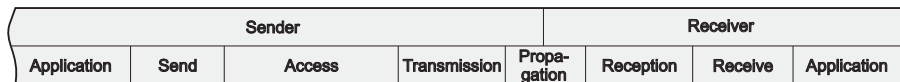
Figure 3.3: The sources of delay in a packet exchange are divided between both the sender and receiver nodes.
