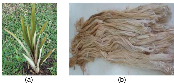
Figura 13. (a) Planta de curauá e (b) fibra de curauá (AMARASEKERA et al., 2009)
