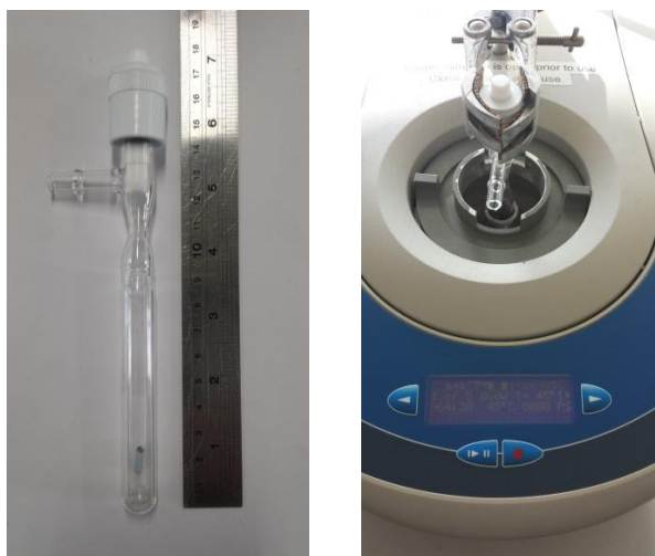
Figure 19: Re-sealable reaction tube and microwave apparatus.
