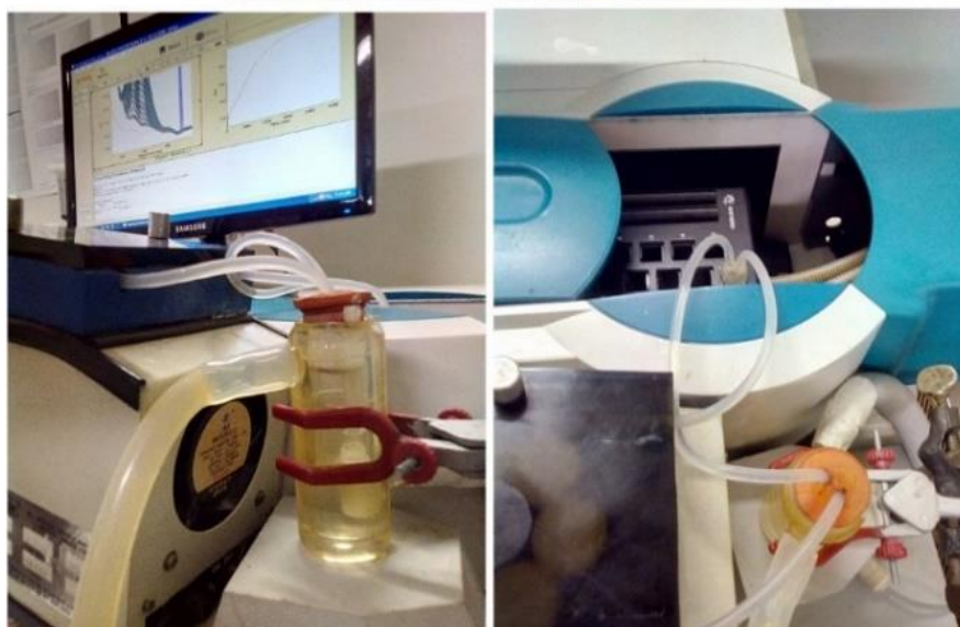
Figure 2. 3. System 1 (reactor) used to monitor the hydrolysis of BDNPP in the presence of the silica materials (PSiM, PSiM-NH 3 + and PSiM-NH 2 La).
