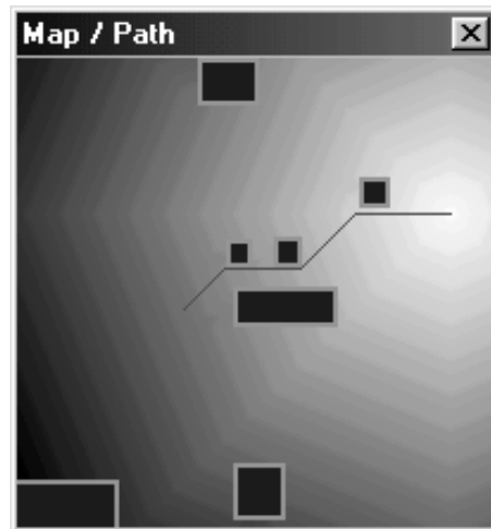
Figure B.3: Map and plan generated using the Grassfire Algorithm.
