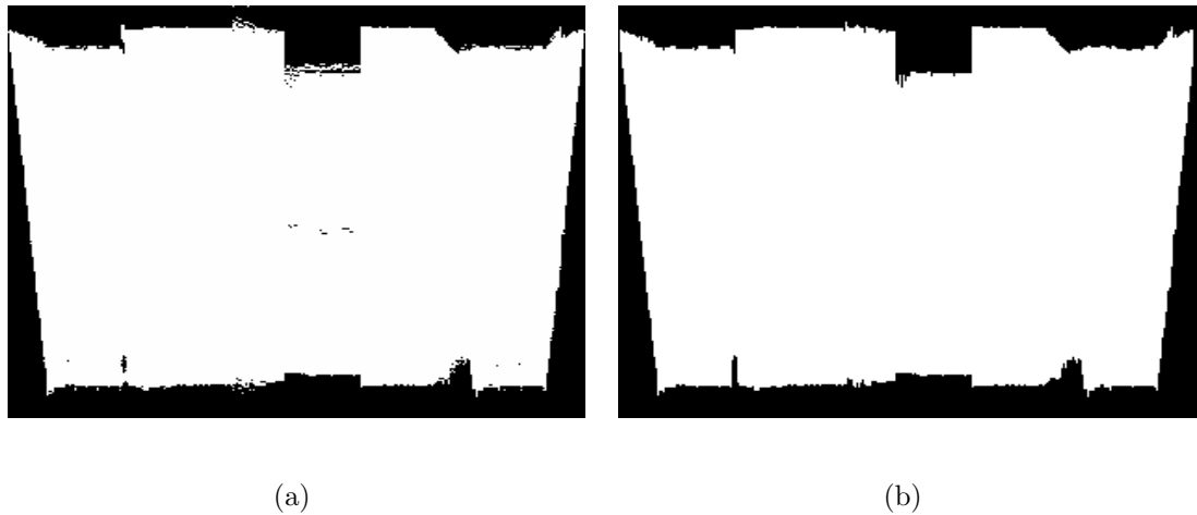
Figure 10.6: Visual rhythm filtered: (a) the thresholded visual rhythm and (b) the result of the morphological filtering (opening followed by a closing). The vertical size of the structuring element is 13.
