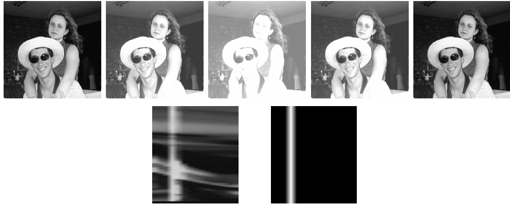
Figure 8.2: Flash video detection: (a) some frames of a sequence with the flash presence; (b) visual rhythm by sub-sampling; (c) detected flash.
