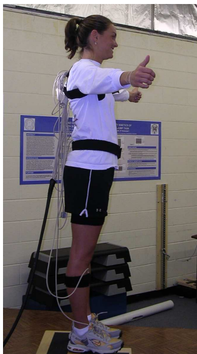
Figura 1.3. Sistema Magnético — Flock of Birds (Ascension Technology Corporation, 2009).
