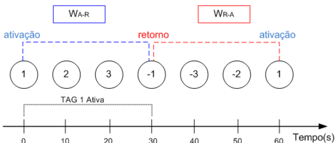
Figura 6 - Janelas W A-R e W R-A do Algoritmo Cross-effect Test de KORDIC et al. 2008 [13]
