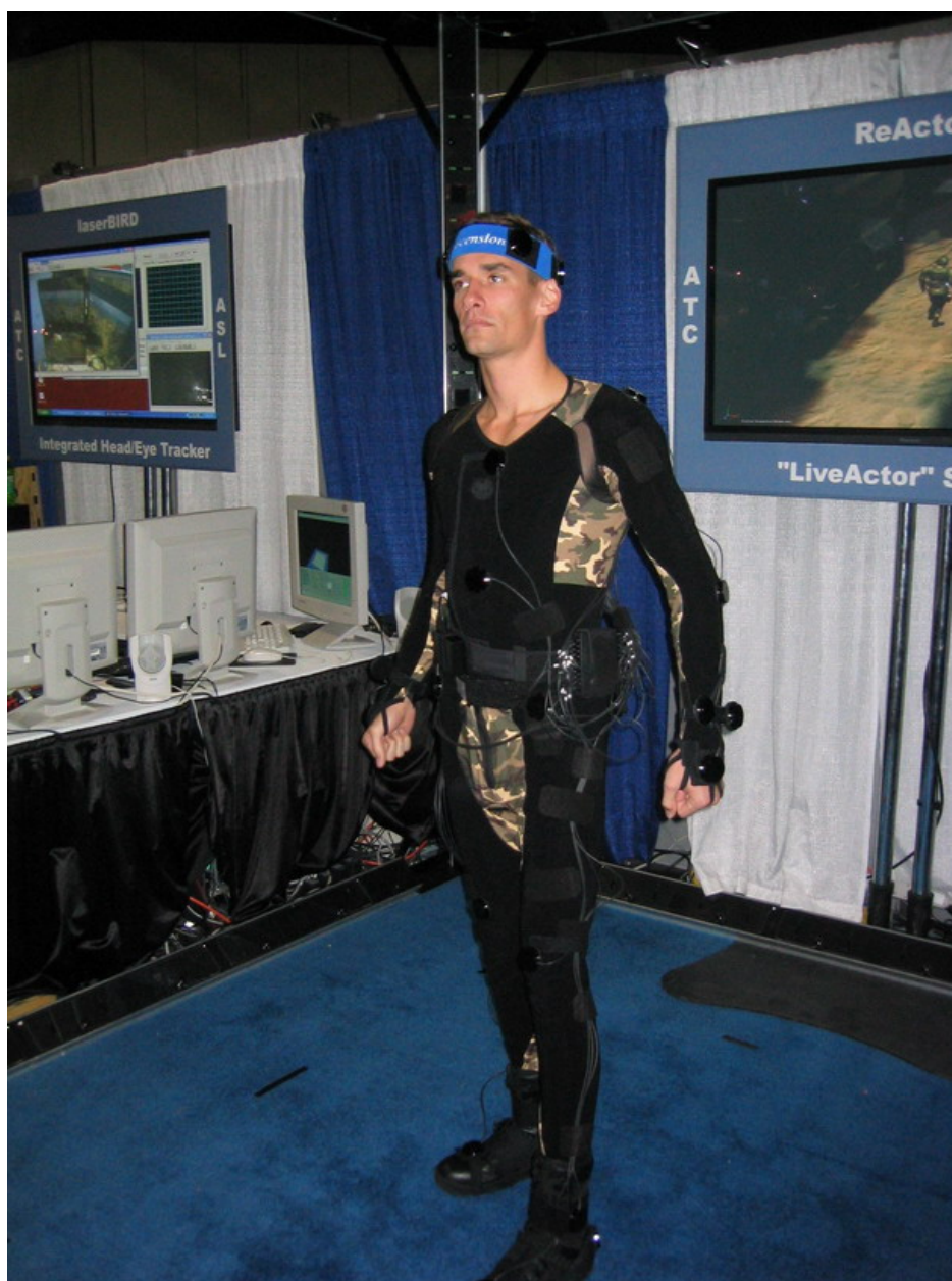
Figura 1.4. Sistema magnético — ReActor 2 [Ascension Technology Corporation, 2010].
