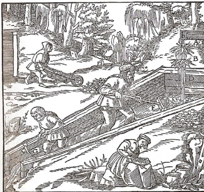
A—LAUNDER. B—INTERLACING FIR TWIGS. C—LOGS; THREE ON ONE SIDE, FOR THE FOURTH CANNOT BE SEEN BECAUSE THE DITCH IS SO FULL WITH MATERIAL NOW BEING WASHED. D—LOGS AT THE HEAD OF THE DITCH. E—BARROW. F—SEVEN-PRONGED FORK. G—HOE
