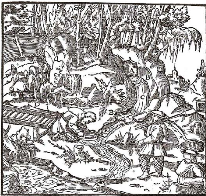
A—GULLY. B—DITCH. C—TORRENT. D—SLUICE BOX EMPLOYED BY THE LUSITANIANS.
