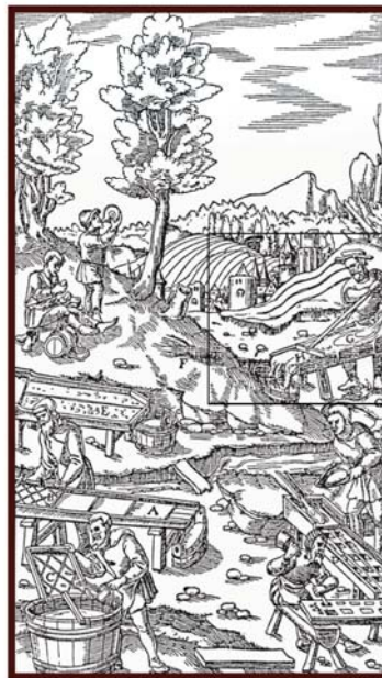
A—SLUICE COVERED WITH CANVAS. B—ITS HEAD FULL OF POCKETS AND GROOVES. C—HEAD REMOVED AND WASHED IN A TUB. D—SLUICE WHICH HAS SQUARE POCKETS. E—SLUICE TO WHOSE PLANKS SMALL SHAVINGS CLING. F—BROOM. G—SKINS OF OXEN. H—WOODEN SCRUBBER.
