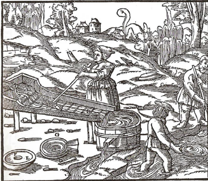
A—HEAD OF THE SLUICE. B—RIFFLES. C—WOODEN SCRUBBER. D—POINTED STICK. E—DISH. F—ITS CUP-LIKE DEPRESSION. G—GROOVED DISH.
